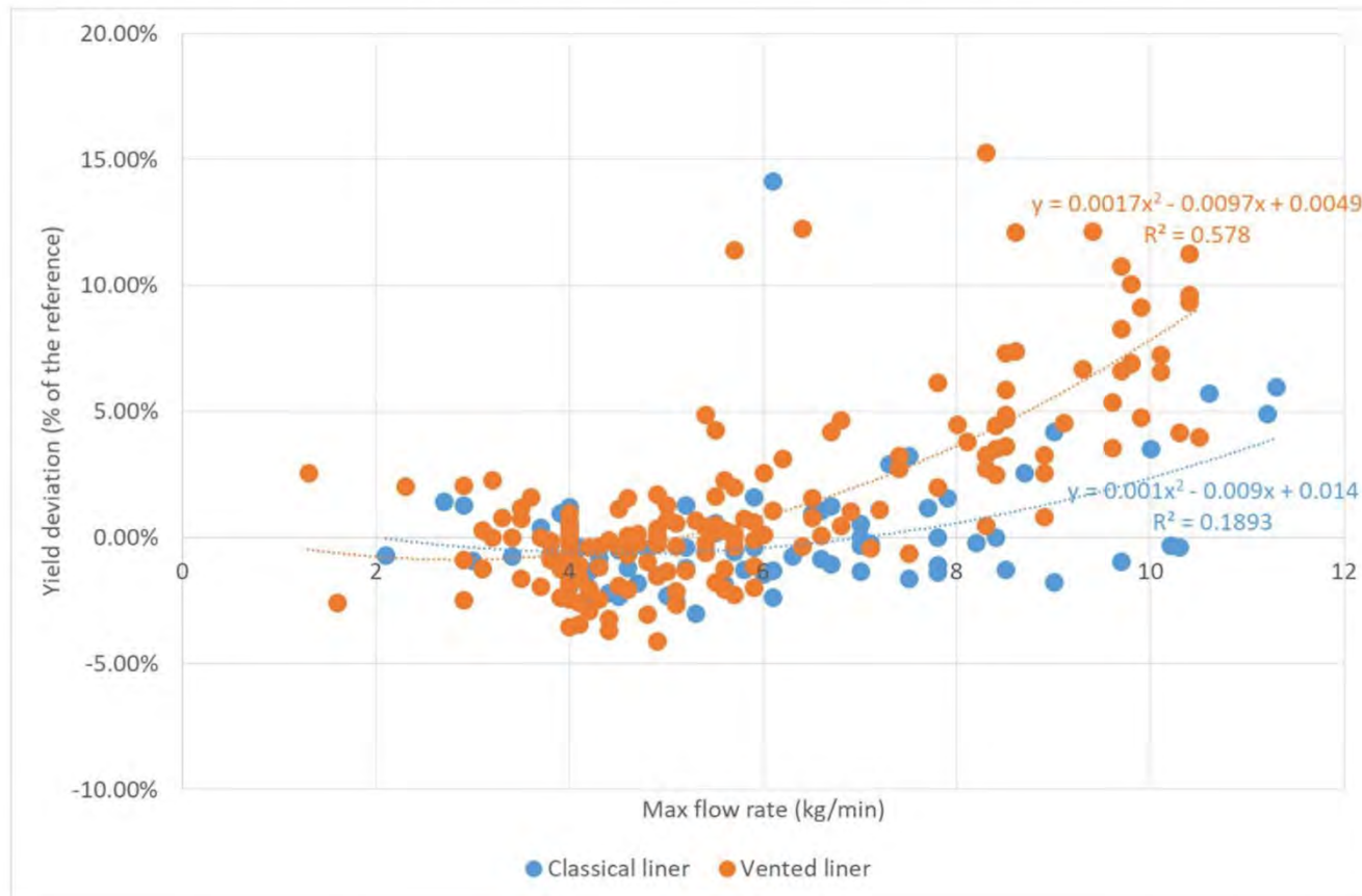
Figure 1: influence of the maximum flow rate on milk yield deviation with classical and vented liners.
